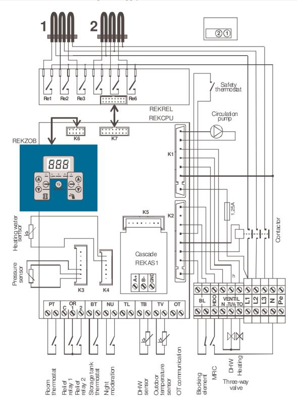
◆ Therm EL 23 boiler connection to the power supply
