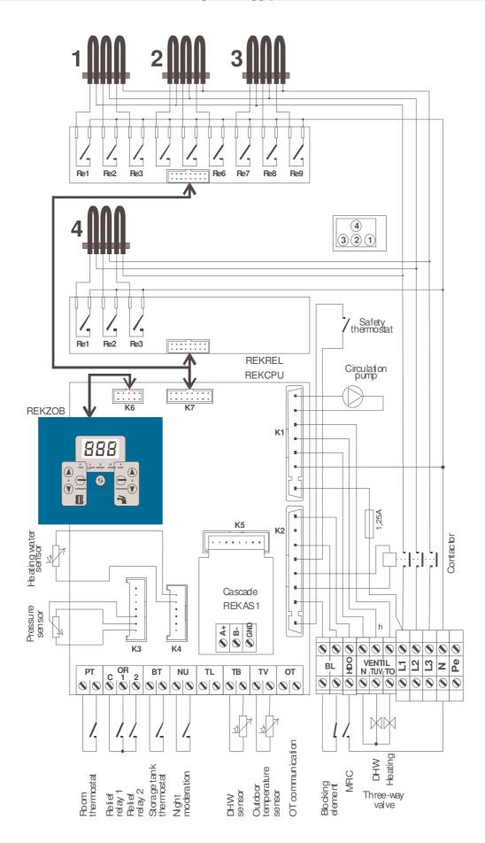
◆ Therm EL 38 boiler connection to the power supply
