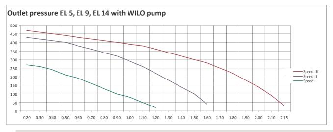
• Min. flow at thermal gradient 20°C
